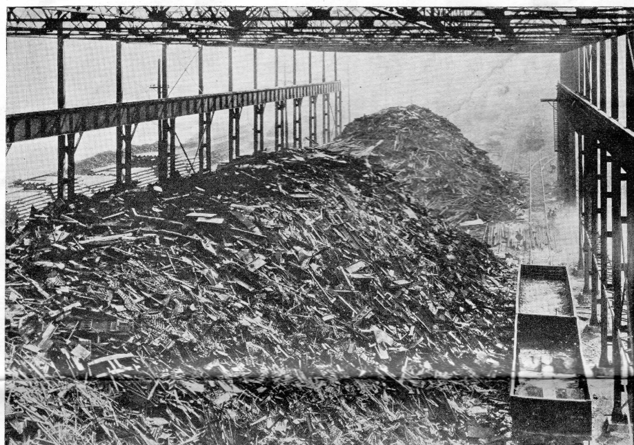
Hundreds of tons of unsegregated iron and steel scrap in this pile. Note comparative size of 50-ton cars at right. (Ewing Galloway photo)
