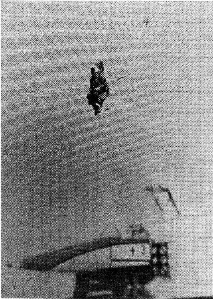
Ejection-system test: Rockets propel the cockpit and pilot down the track; pilot ejected from aircraft cockpit; parachutes deploy for the pilot and ejection system.
